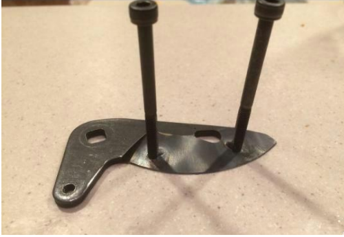
Figure 35. Welded Bolts to Blade.
