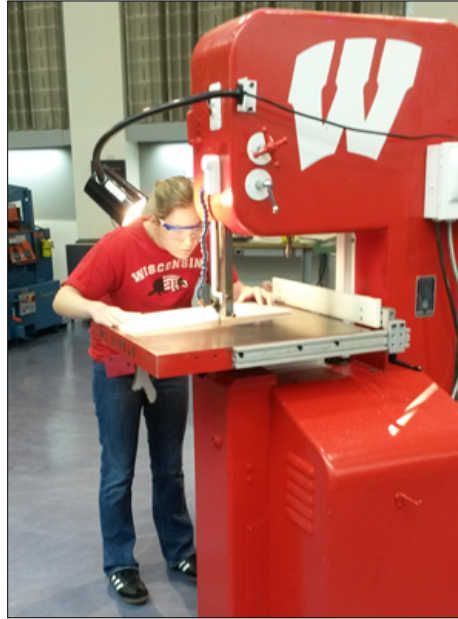
Figure 29. Cutting the Plastic Sheet with Bandsaw
