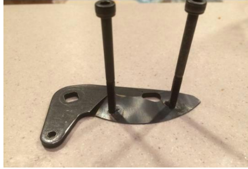
Figure 14. Screws in the blade. This is a picture of the two screws in the blade of the arm cutter. At the top of the screws is where the rubber bands are placed.
